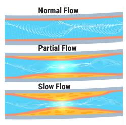
This phenomenon can be explained using a water pipe analogy, the flow rate of water through the pipe is constant, much like the current through a cell string. When there is mismatch among panels, this is like a water pipe getting partially blocked and flow rate of water through this pipe becomes slower, and it affects the flow rate of all other pipes connecting to it. Similarly, the current through the entire string will reduce when there is mismatch
